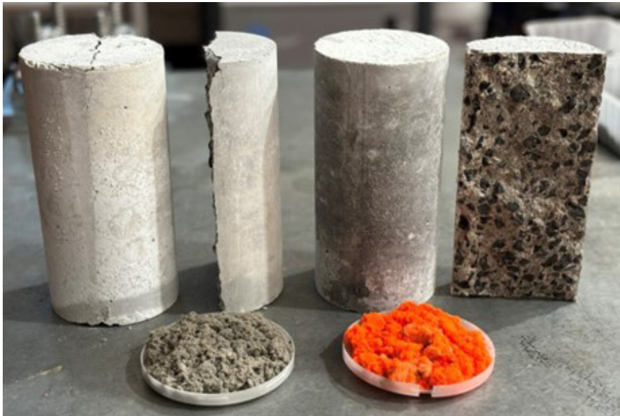
Hi-vis vest textile polyester fibers (front-right), cardboard fibres (front-left), and concrete specimens made with these (back row).
