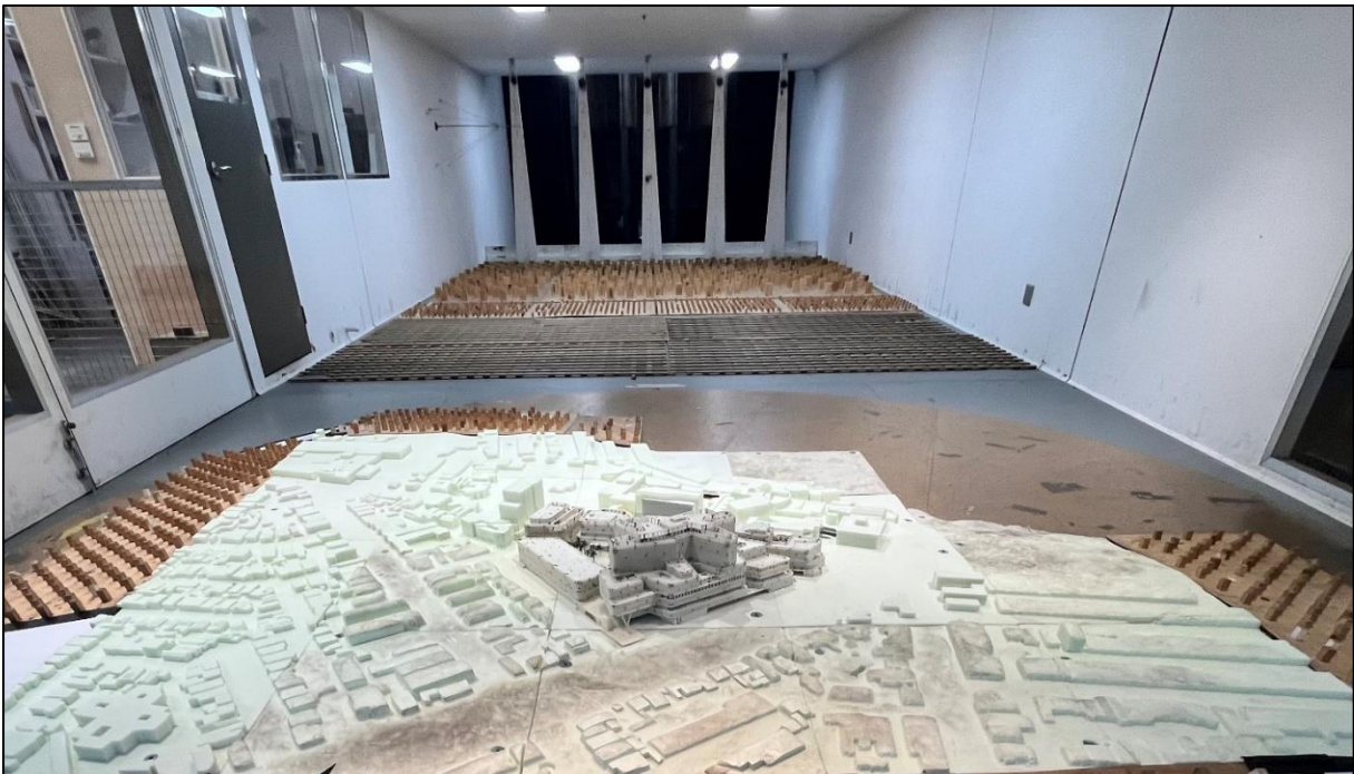
Figure 2a - View from the south of the 1/300 scale model of the proposed VU CHTF Development in the wind tunnel.
