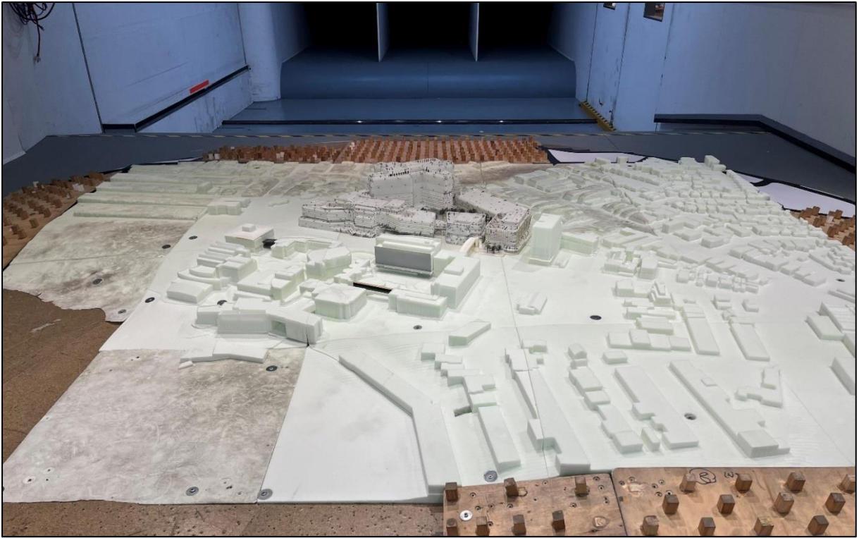
Figure 2b - View from the south of the 1/300 scale model of the proposed VU CHTF Development in the wind tunnel.
