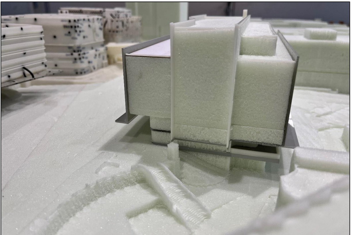
Figure 2c - Close-up view from the south of the 1/300 scale model of the proposed VU CHTF Development in the wind tunnel.
